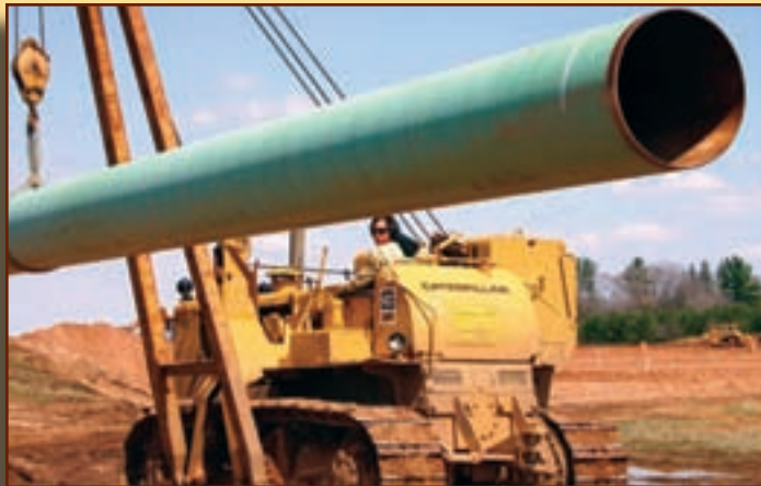
A Local 49 pipeline trainee at the local's training center in Hinckley, MN practices maneuvering massive pipes into a ditch with a sideboom.
